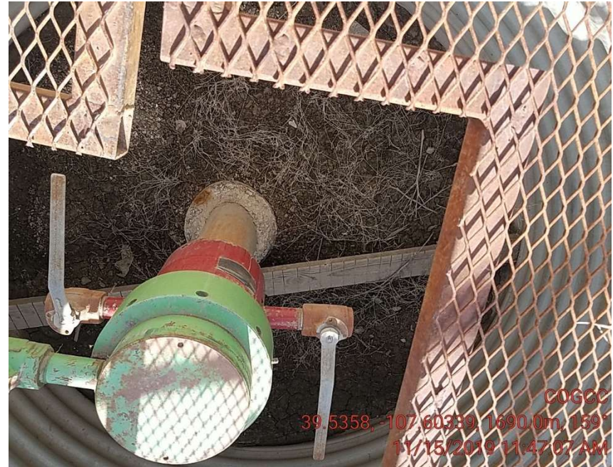
Wildlife escape board not positioned
