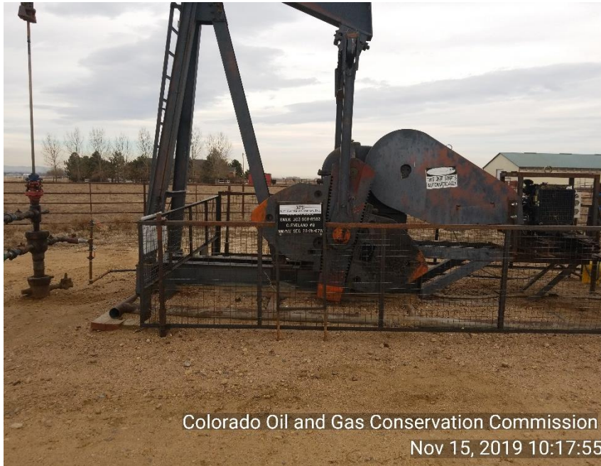
Photo1 Well head and PU
