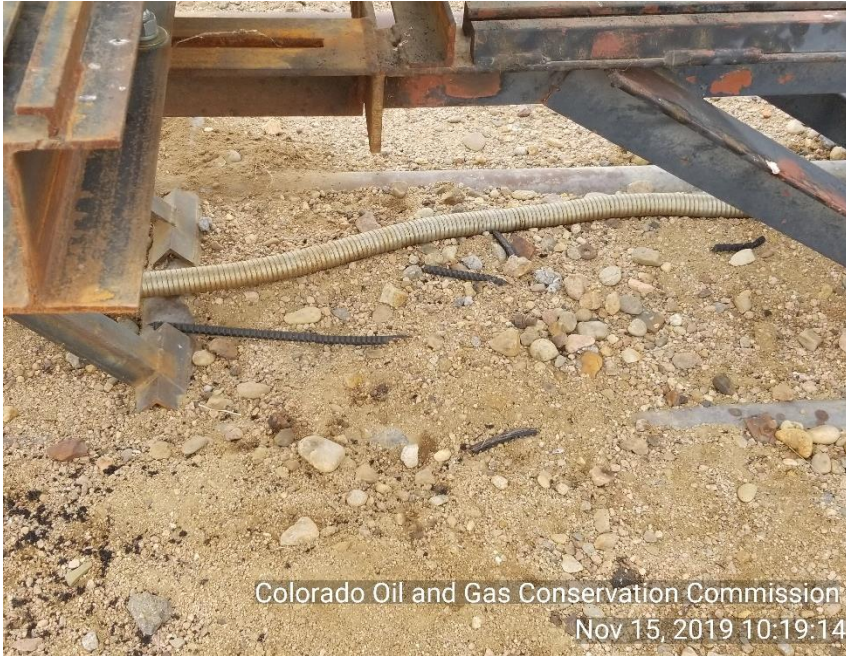
Photo 5 Mechanical issue: PU motor belt appears to be in pieces and laying on ground. PU is not operable.
