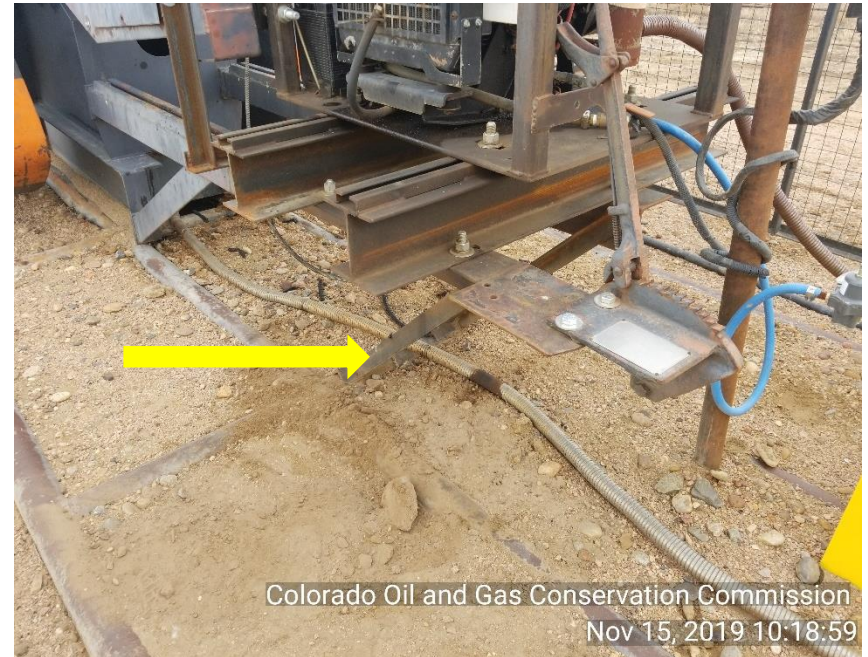
Photo 4 Stained soil under PU motor. Mechanical issue: PU motor appears to be leaking.
