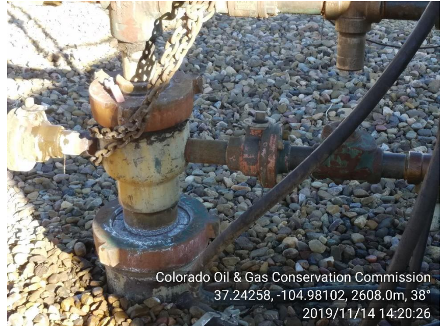
PHOTO 4: AREA OF IMPACTED SOIL AROUND WELLHEAD. Remove and dispose impacted material in approved manner, service and maintain equipment and self inspect to prevent recurrence of conditions per 1002.f(2) and 907. CA DATE 12-14-19.
