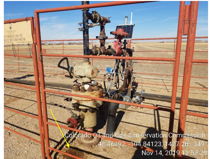
Photo 10: Wellhead/stained soil
