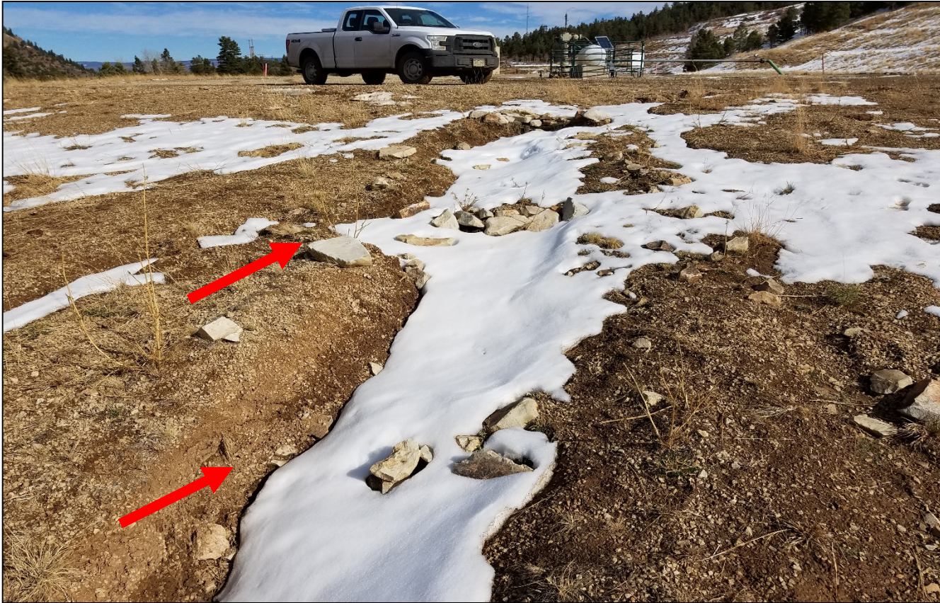
Photo 6. The above photo shows the erosion channel and check dams which have failed.
