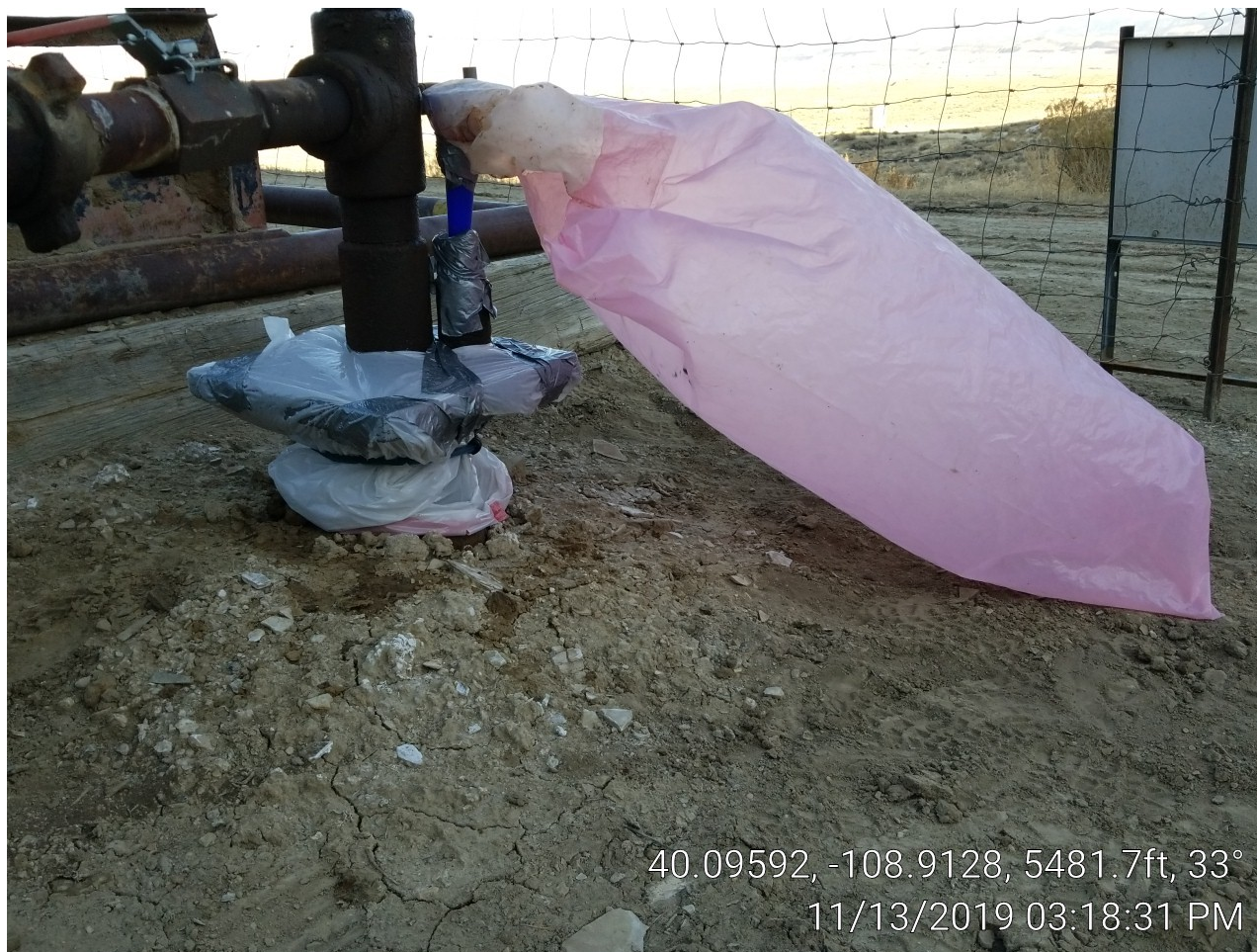
Photo 3. Well head with gas collection bag attached.
