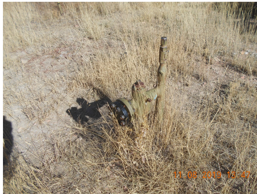
Flowline riser with blind flange. Blowdown pit.
