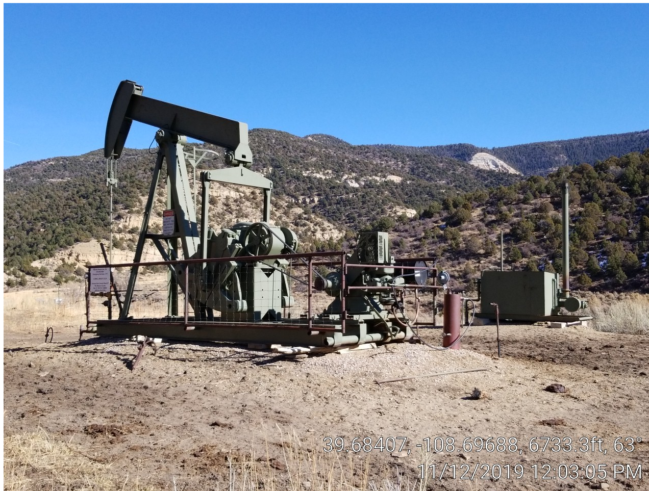
Photo 1. Pump jack and separator.
