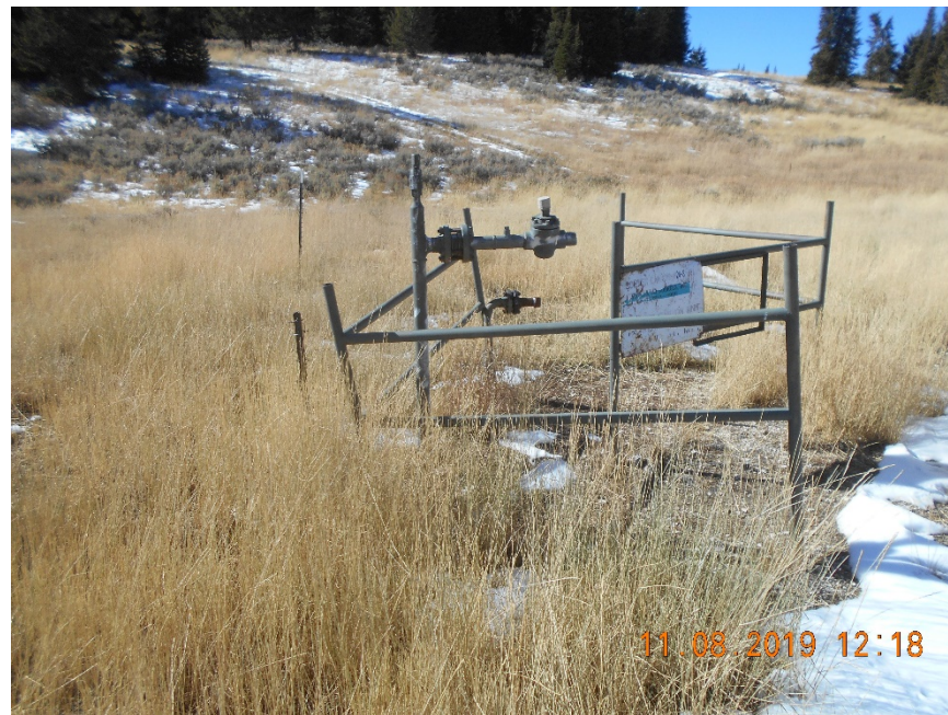
Flowline riser with fence. Dissconnected.
