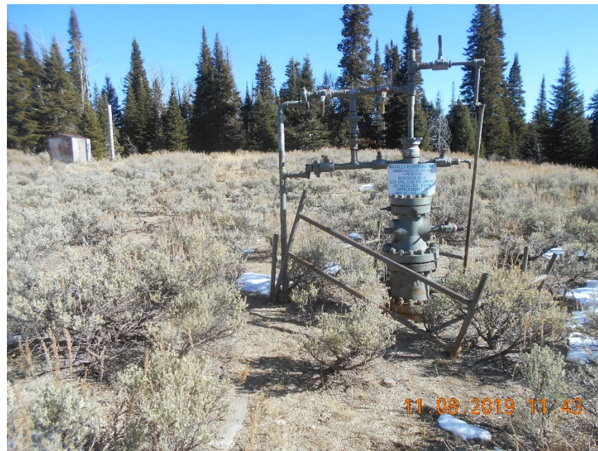
Wellhead with sign. Pipe fence sections down.
