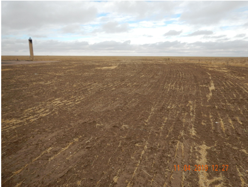
Photo 1. Photo taken from the eastern interim area, facing North. Photo illustrates Operator has performed interim reclamation to reduce areas only needed for production operations per Rule 1003. Note: Appears straw mulch was crimped as an erosion control but has already blown off location which will not ensure the seeded soil is stabilized. COGCC staff would recommend re-installing erosion controls and using long-fiber weed-free mulch.
