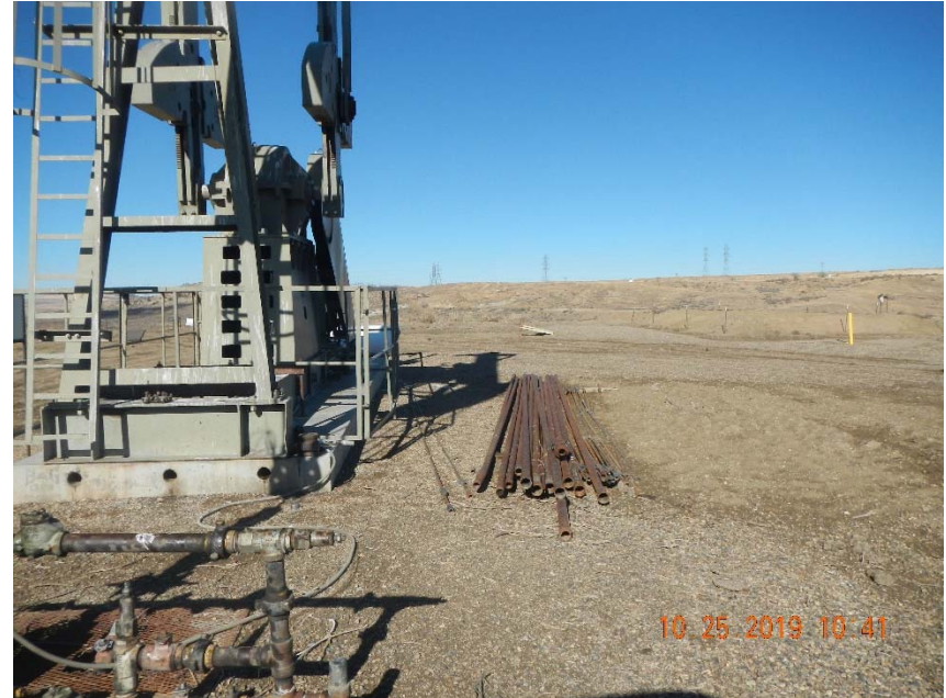
Photo 2. Tubing stored at wellhead.
