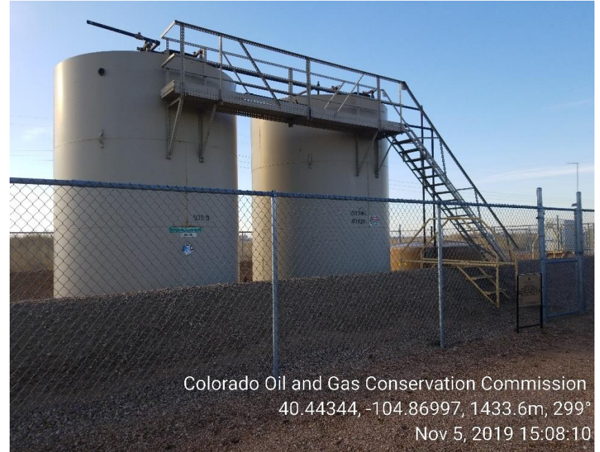
Photo 2: Tank Battery; inadequate berm
