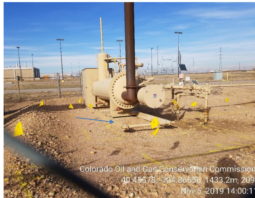
Photo 8: Separator NOT anchored
