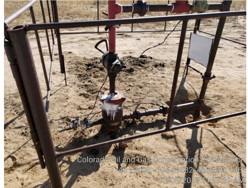
Photo #3 No Active leak at the casing collar. On 11/5/19
