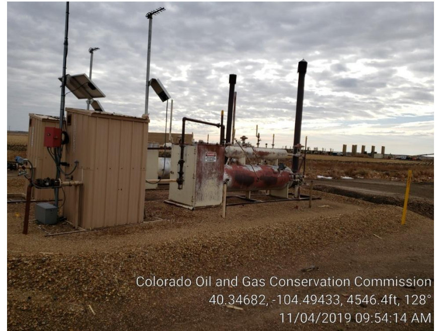
Photo #3 Separator & Meter Run
