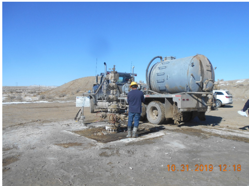
Injection wellhead.
