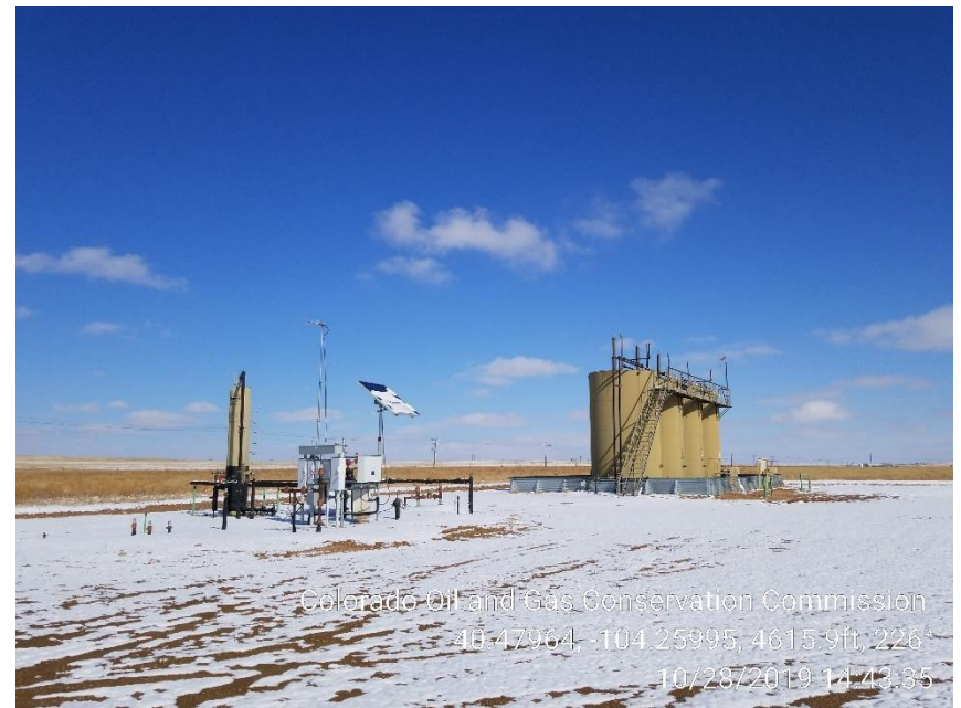
Photo 2 – Tank Battery
