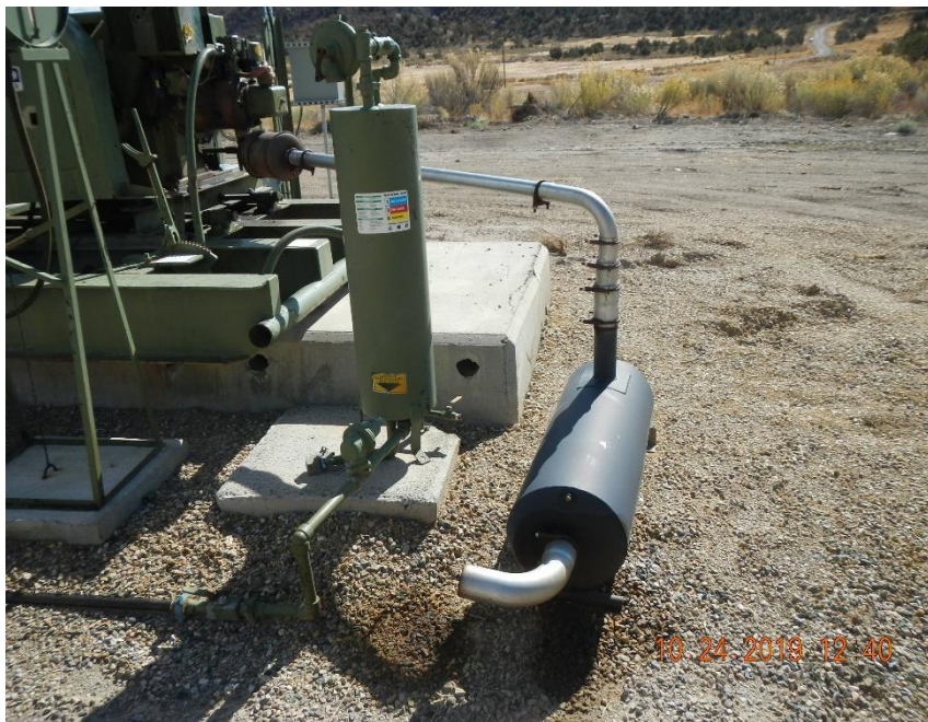
Stained gravel at exhaust outlet for prime mover.
