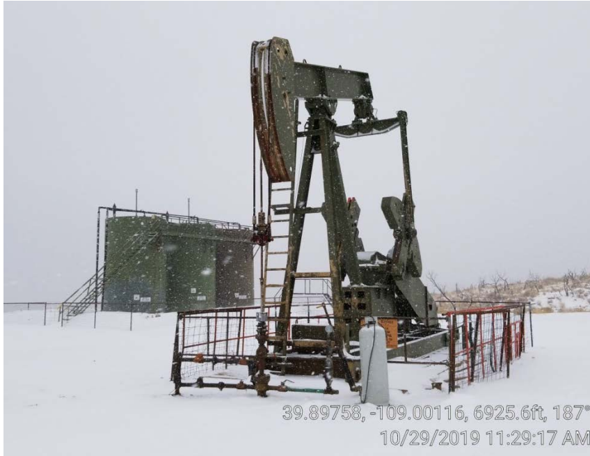
Photo 2. Pump jack & tank battery.
