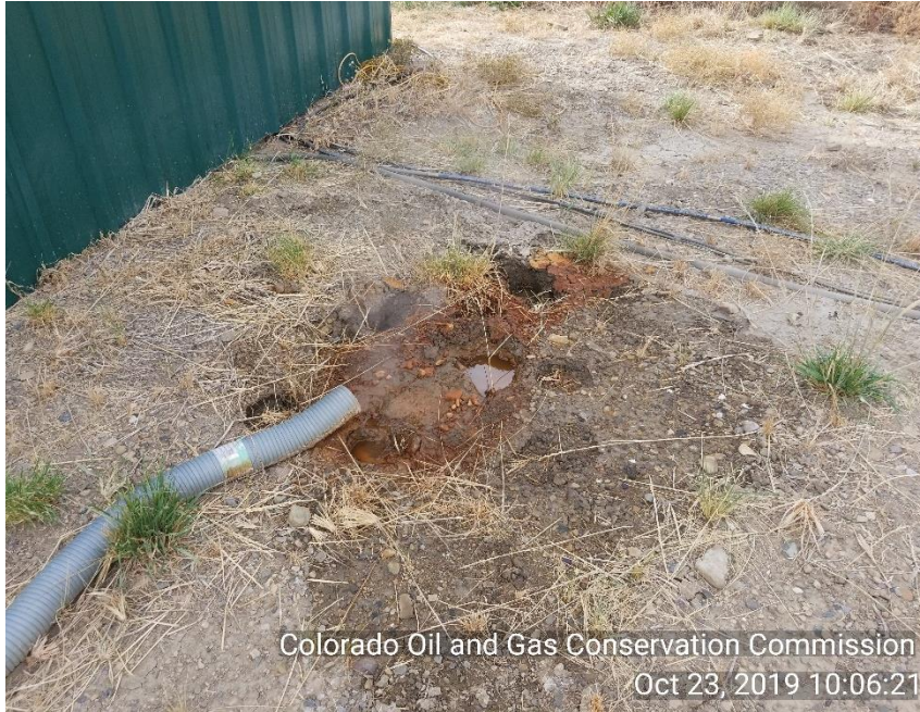
Photo 5 Stained soil from HYD motor exhaust pipe.
