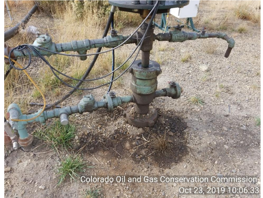
Photo 6 Mechanical issues and stained soil around well head
