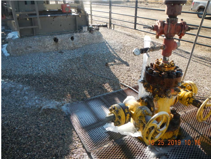
Photo 1. Ongoing leak at wellhead.
