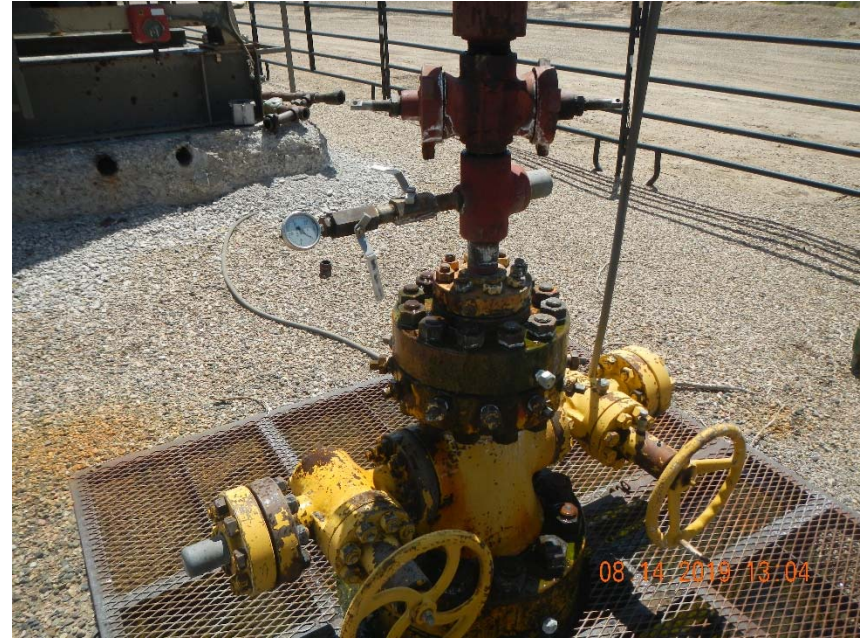
Photo 2. Ongoing leak at wellhead. Photo from 8/14/2019 inspection document number 689802979.
