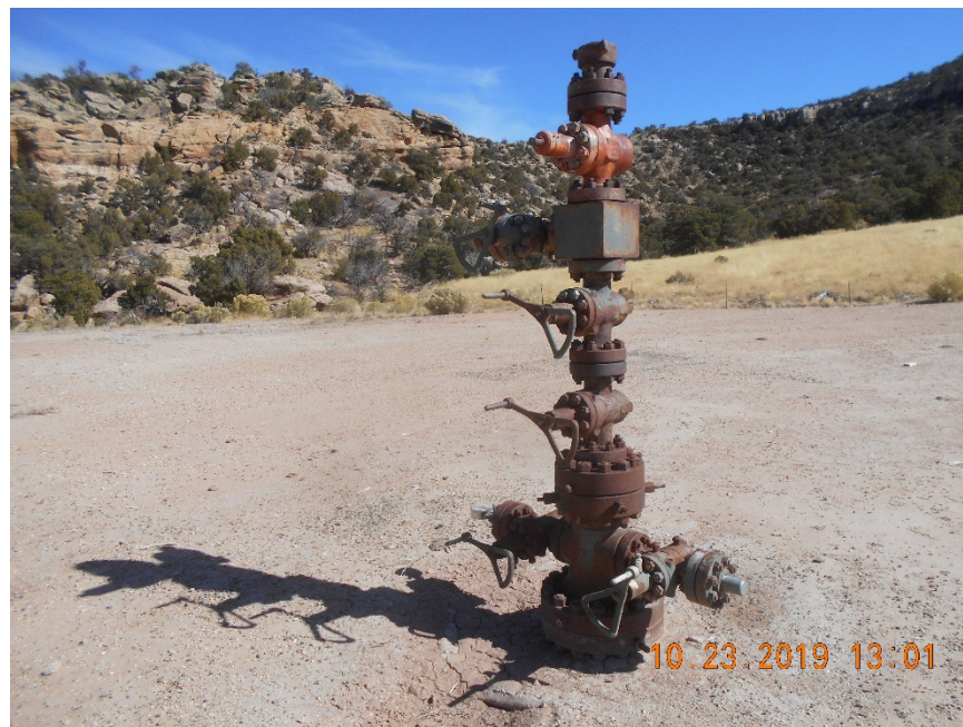
Temporarily Abandoned Wellhead
