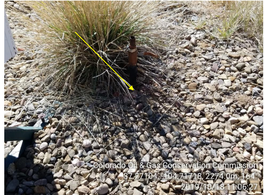
PHOTO 6: UNUSED EQUIPMENT UNUSED UNMARKED 1" RISER. REMOVE ALL UNUSED RISER IN ACCORDANCE WITH NTO. CA DATE 12-18-19
