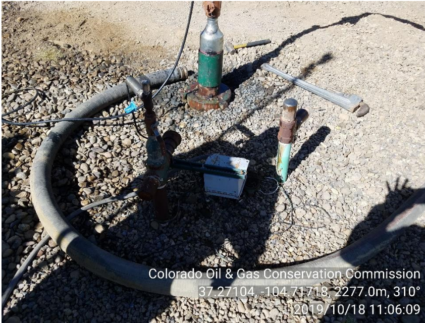
PHOTO 5: UNUSED EQUIPMENT UNUSED UNMARKED RISERS. REMOVE ALL UNUSED RISER IN ACCORDANCE WITH NTO. CA DATE 12-18-19
