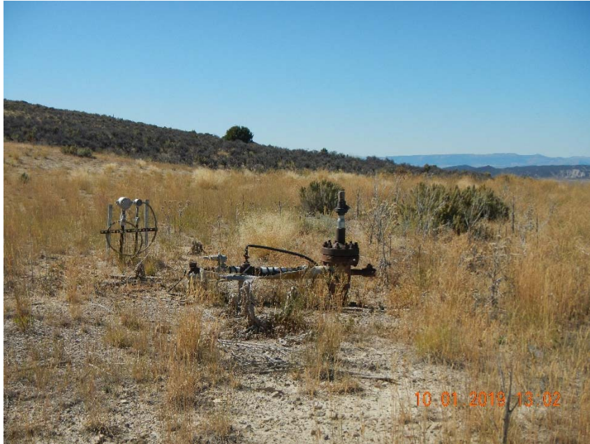
Photo 2. No wellhead sign. Unmarked risers at wellhead. Weeds on location.
