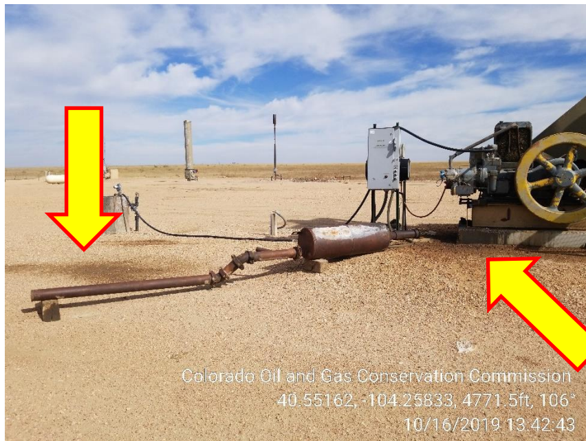
Photo 3 – Stained Soil at Exhaust and Engine
