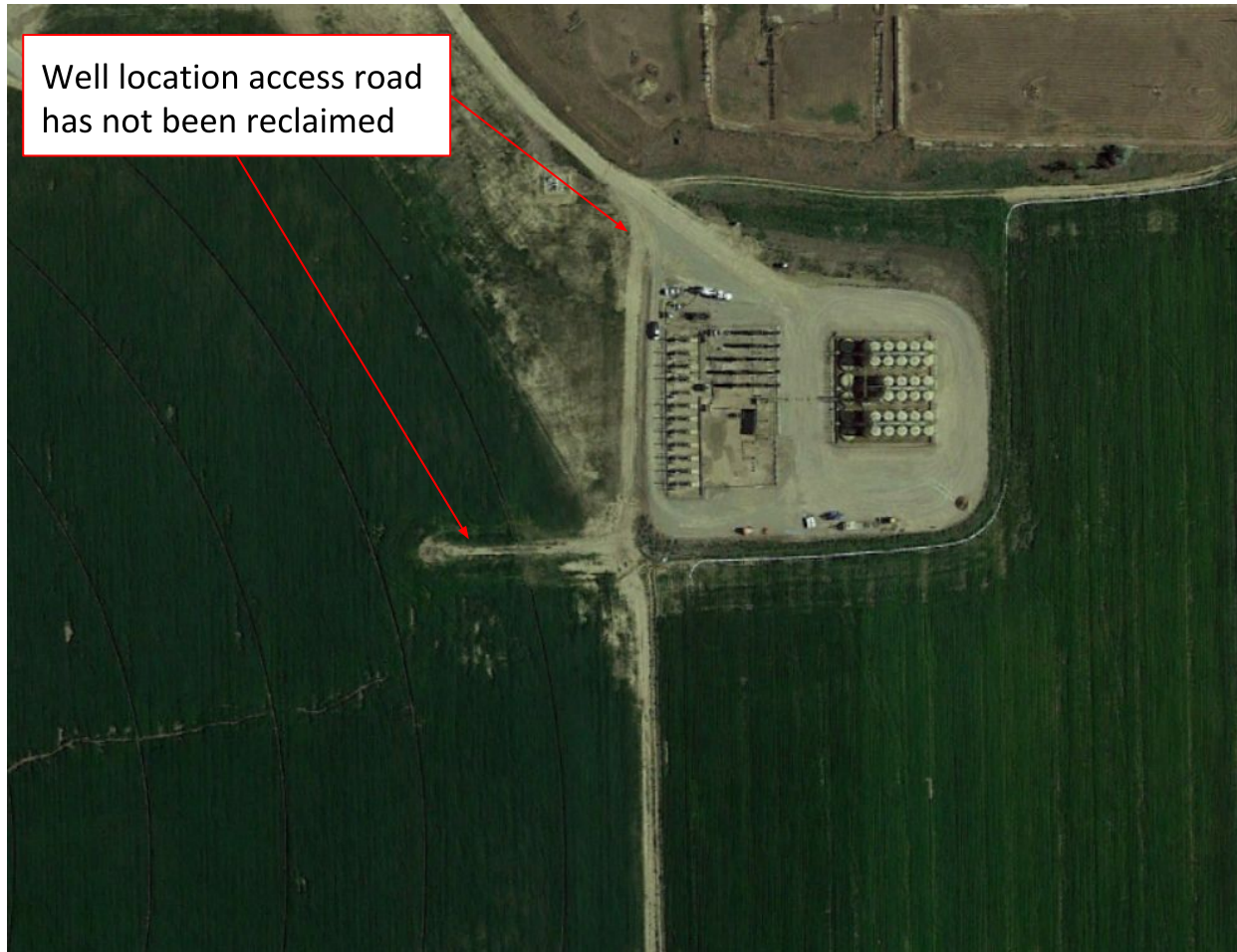
Photo 2. Google Earth aerial photo taken 5/31/2018, approximately 3 months prior to plugging operations. At the time of this inspection, the well location access road has not been reclaimed.
