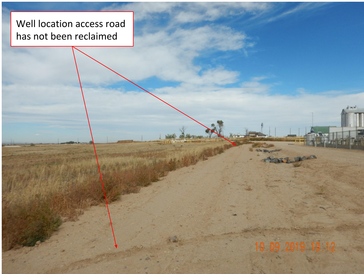
Photo 4. Photo taken from the southern well location access road, facing North. Operator has failed to properly recontour and reclaim the well location road.
