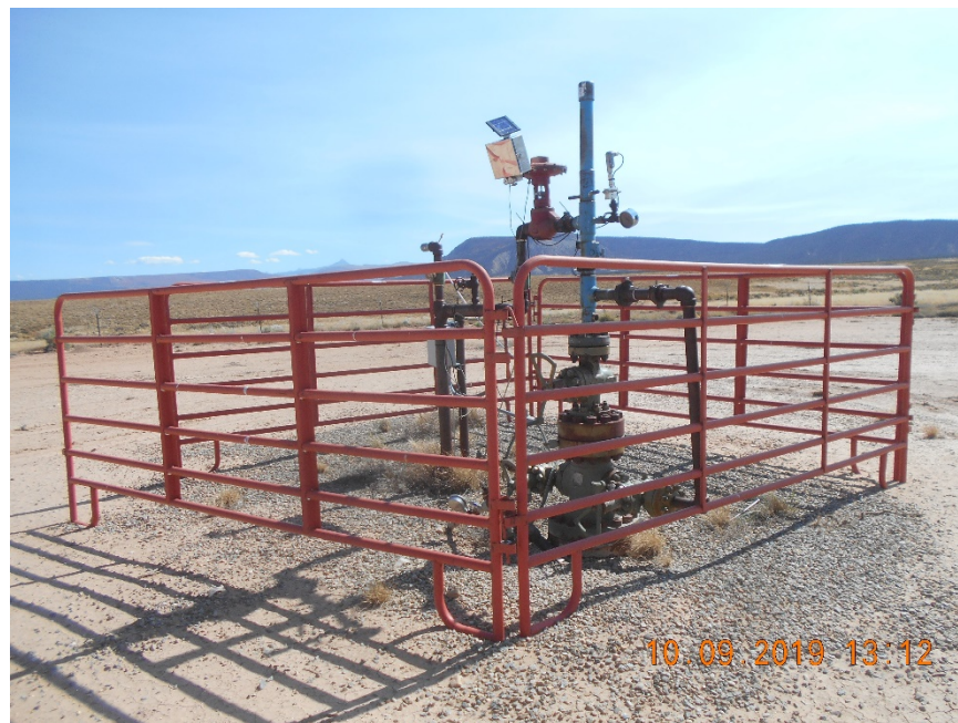
Wellhead with fencing
