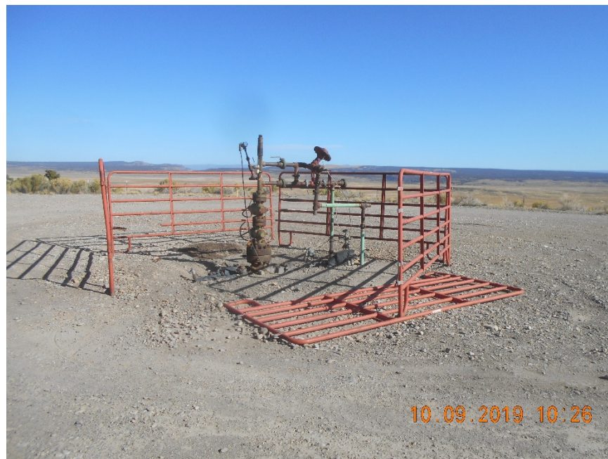
Wellhead with fencing
