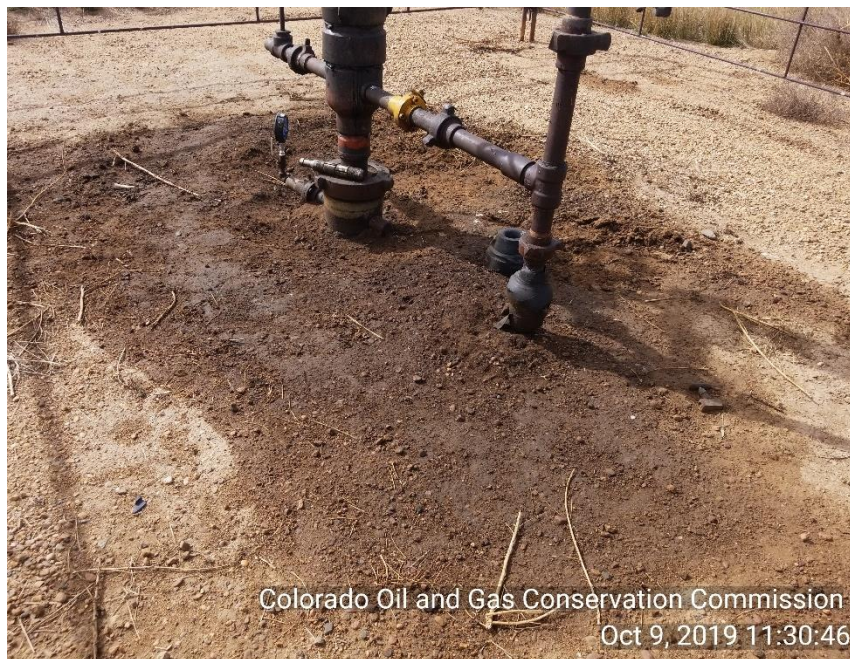
Photo 3 Stained soil around Well head
