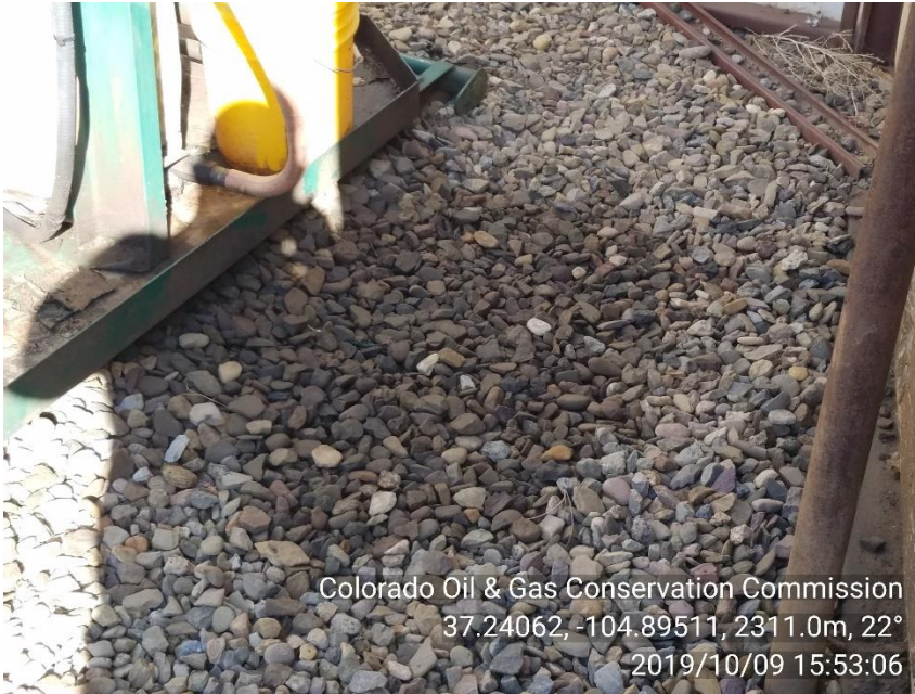
PHOTO 3: AREA OF IMPACTED GRAVEL/SOIL NEAR COMPRESSOR. Properly treat or dispose of oily waste in accordance with 907.e. CA DATE 11-9-19
