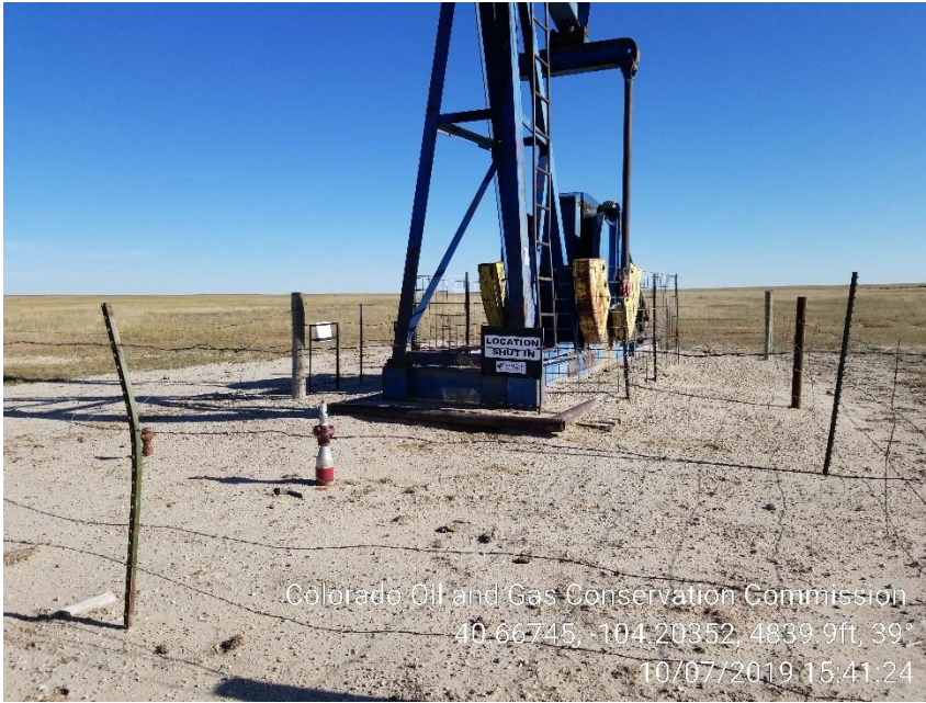
Photo 1 – Pumping Unit and Wellhead TA'd
