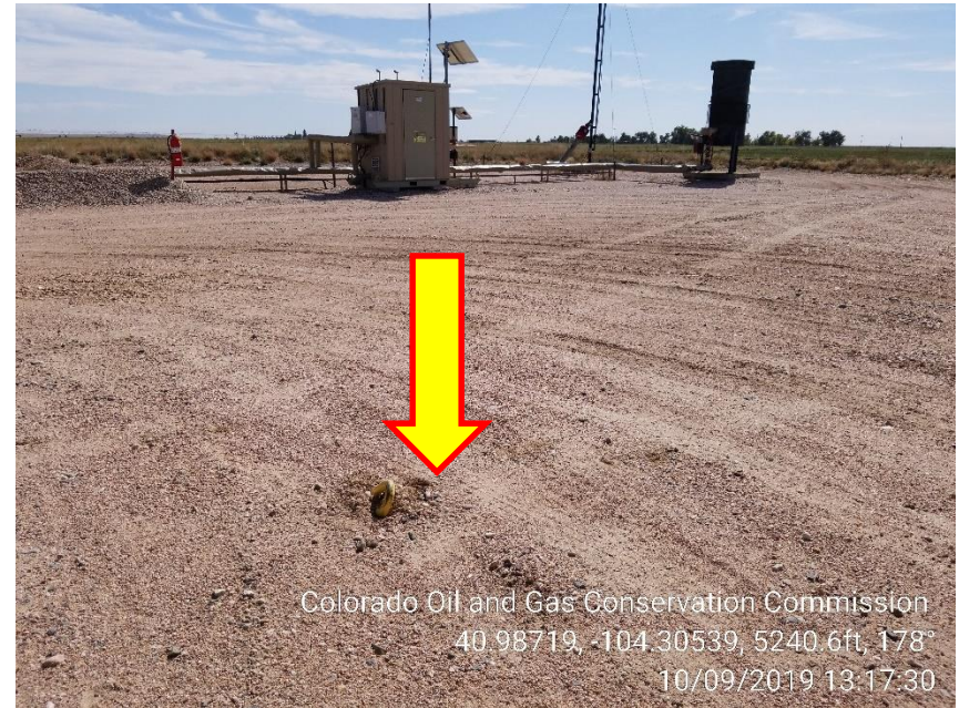
Photo 4 – NE Deadman Anchor not marked
