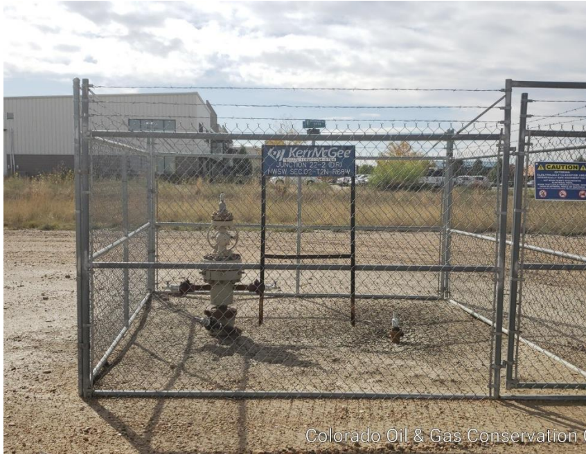
Photo #1 Junction #22-2 WH. Well is TA all production lines removed from WH.
