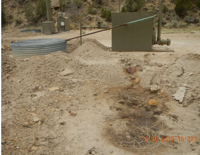
Photo #7 – View of the pit 15 feet by 15 feet by 2 feet deep pit located north of the horizontal heated separator.
