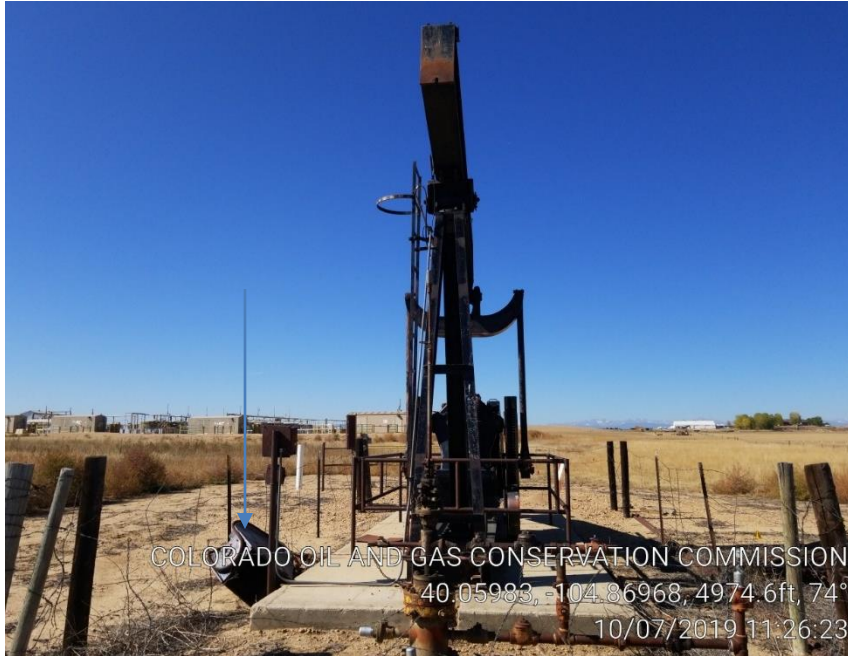
Pic 1 pumping unit not connected to rods/horses head on ground
