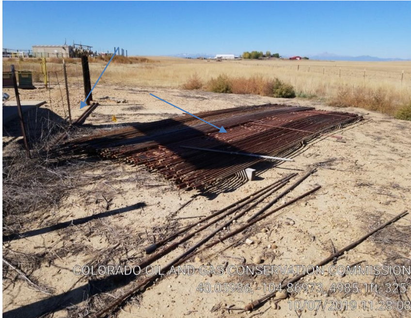
Pic 3 sucker rods, and tubing laying next to pumping unit
