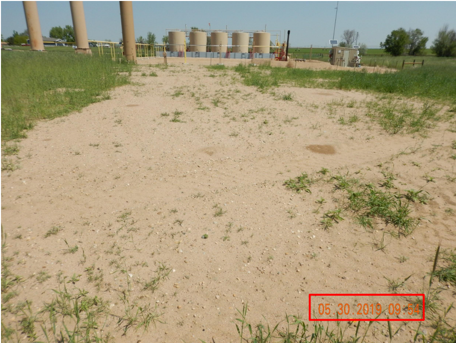
Photo 1. Photo taken from a portion of the flowline area on May 30, 2019, facing North. Photo illustrates a flowline area disturbance that has not been properly reclaimed per Reclamation rules. Photo illustrates bare ground with little, to no, establishment of reference area species.
