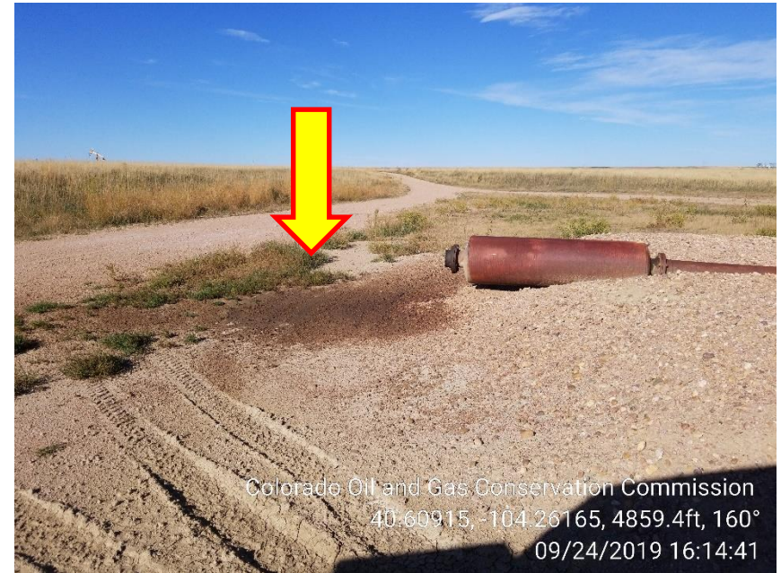
Photo 4 – Stained Soil at Exhaust
