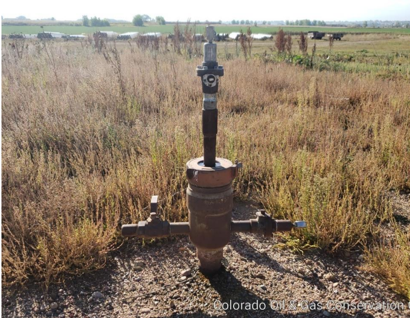
Photo #1 WH doesn't appear TA no flow line connected
