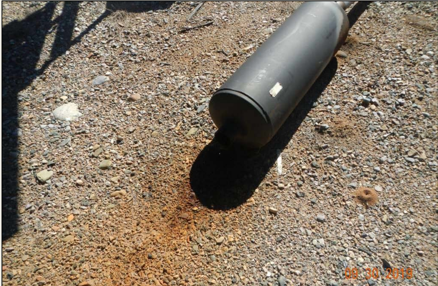
Photo 2. View of oily material on well pad surface. Liquid observed on soil surface. This material is a potential stormwater pollutant.
