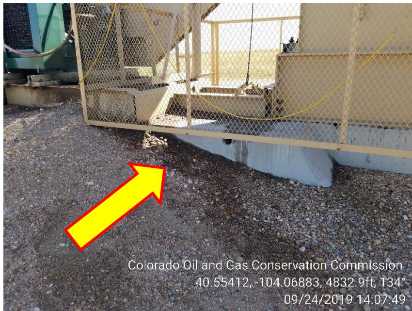
Photo 7 – Stained Soil at the back of the Pumping Unit
