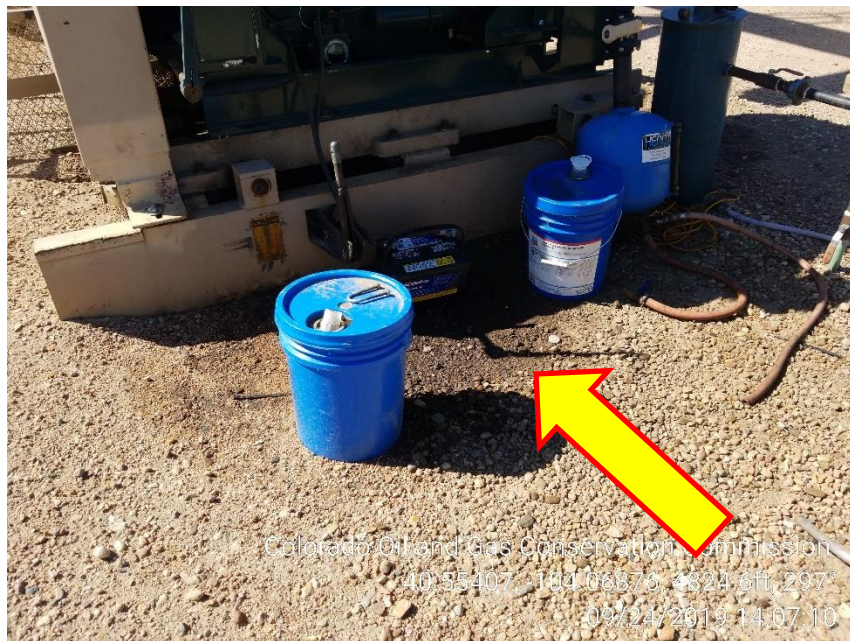
Photo 9 – Stained Soil at the back of the Pumping Unit
