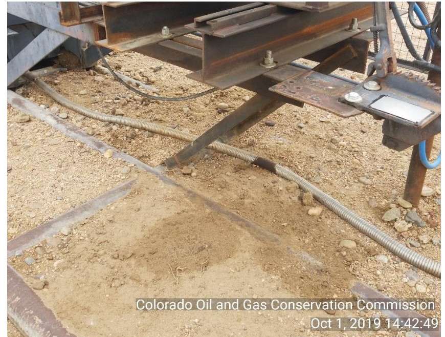
Photo 4 Stained soil under PU motor
