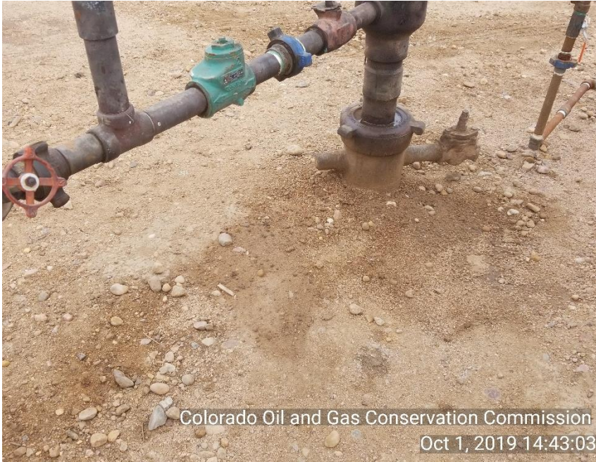
Photo 5 Stained soil around well head.
