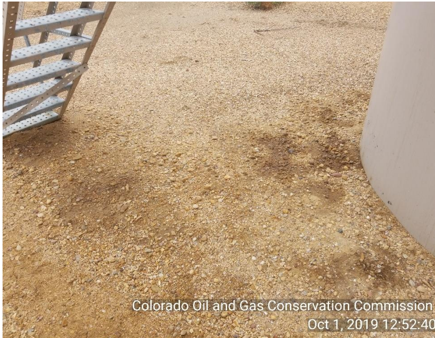
Photo 9 Stained soil around crude oil tank
