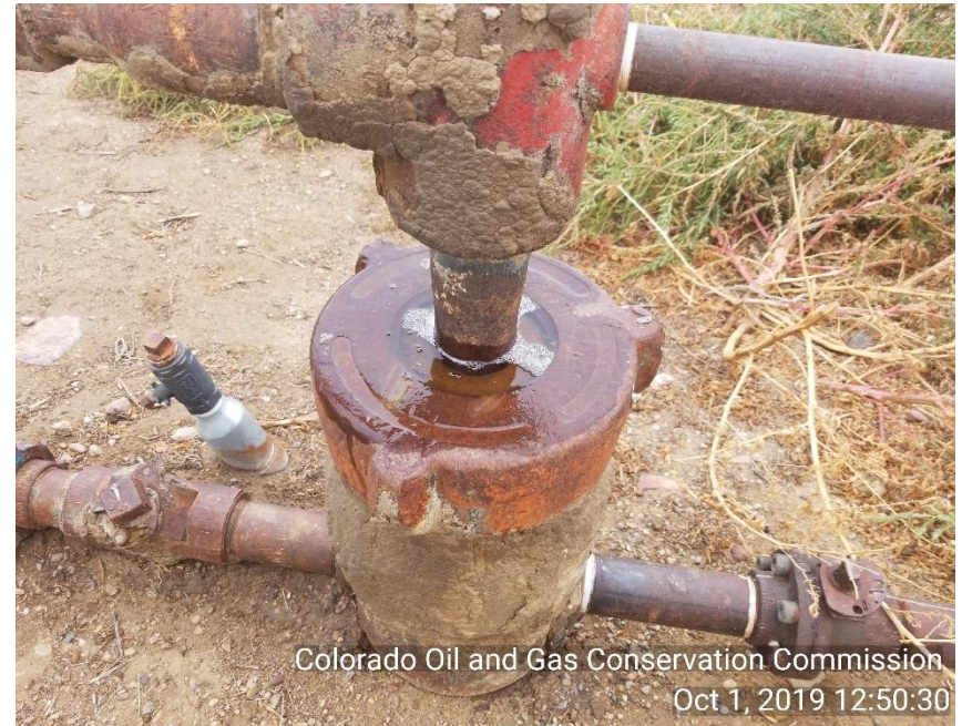
Photo 6 VENTING: bubbles show what appears to be well head leaking at the tubing.
