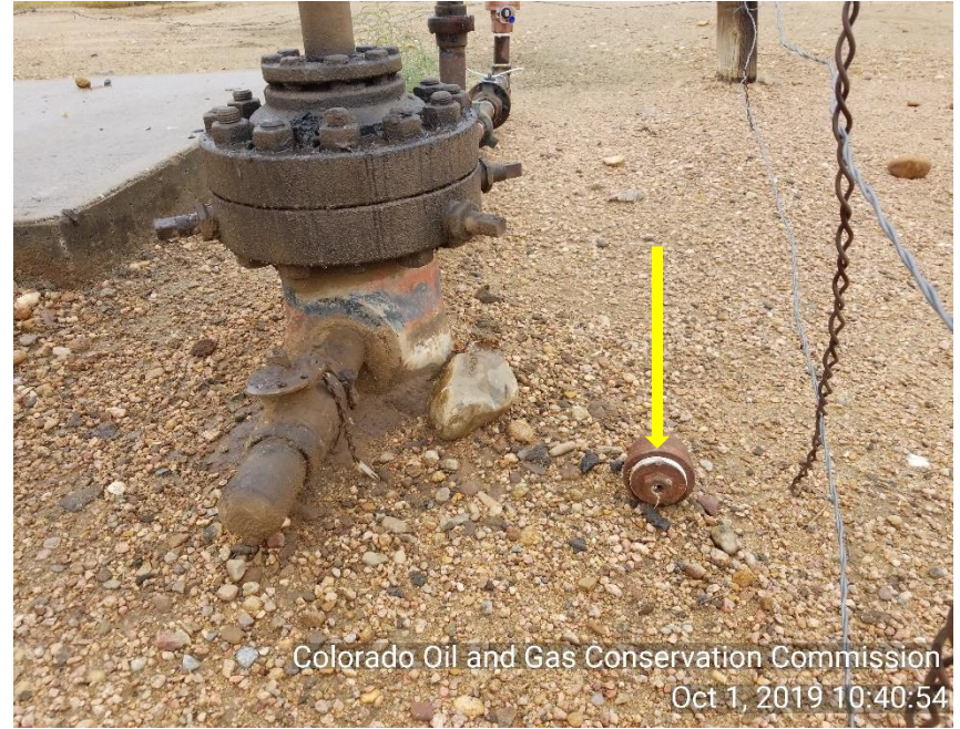
Photo 2 Mechanical issue Braden head 1/4 hole open on 2" bushing.
