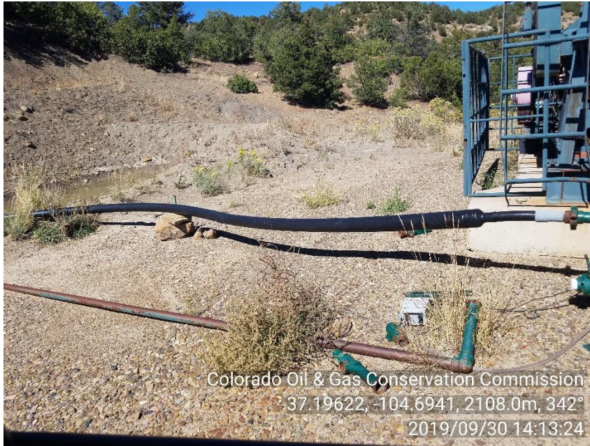
PHOTO 3: UNUSED EQUIPMENT (2" PIPE AND FITTINGS). REMOVE UNUSED EQUIPMENT, COMPLY WITH RULE 603.f. CA DATE 10-30-19
