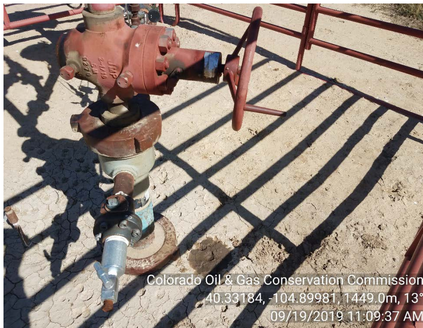
Master valve and stained soil on 9/19/19
