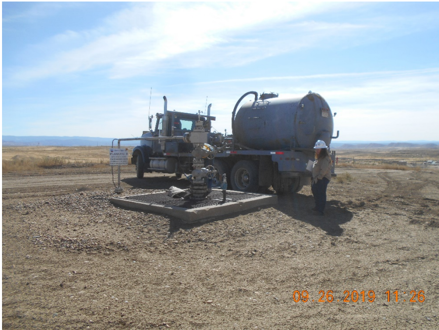
Injection wellhead
