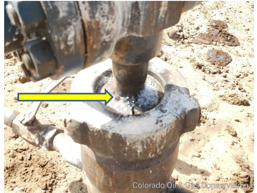
Photo #2 Packing leaking on WH
