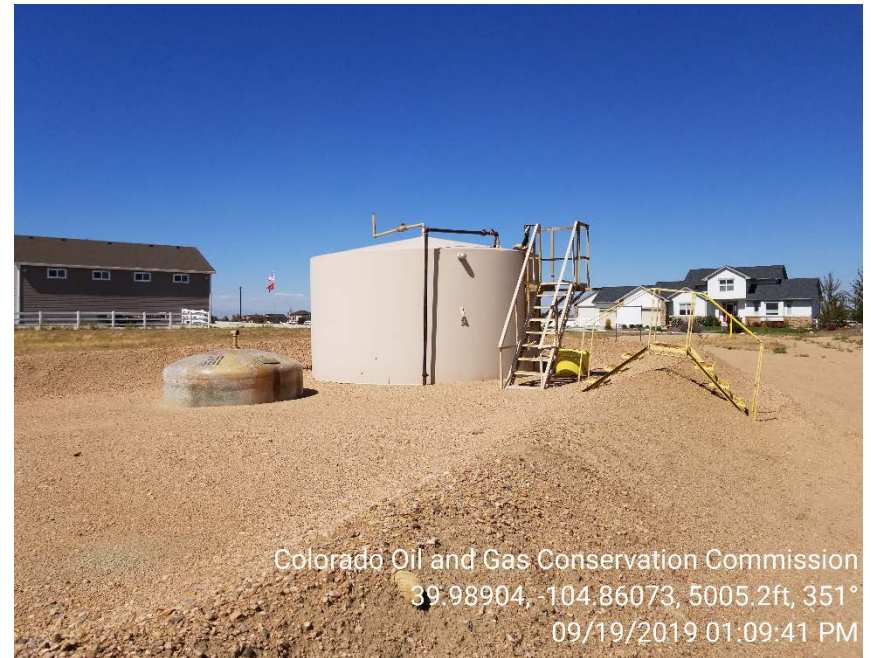
Photo 2 – Location photo; fiberglass partially buried produced water tank on site
