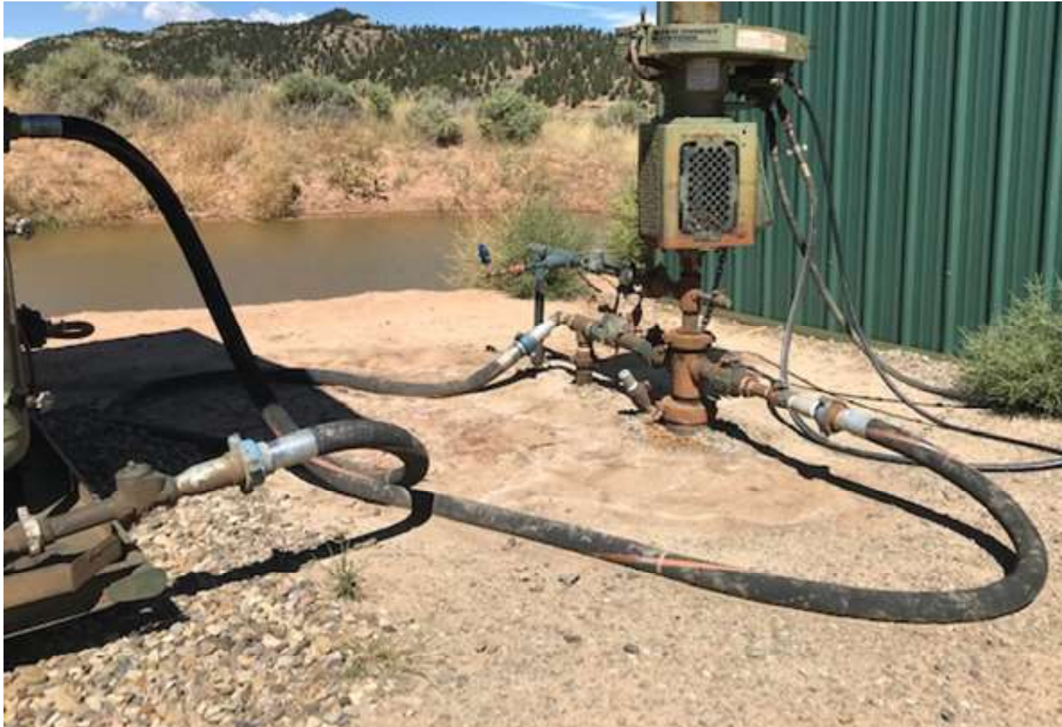
PHOTO 1: Wellhead photo taken on 09/20/19 at 12:19 pm. On 09/19/19 the lease operator found the wellhead packings were leaking. The well was shut in and the packings were repaired. Due to the water level in the production pit the lease operator left the well shut in. The top layer of the soil was scraped up. The soil was dry at the time of inspection.
